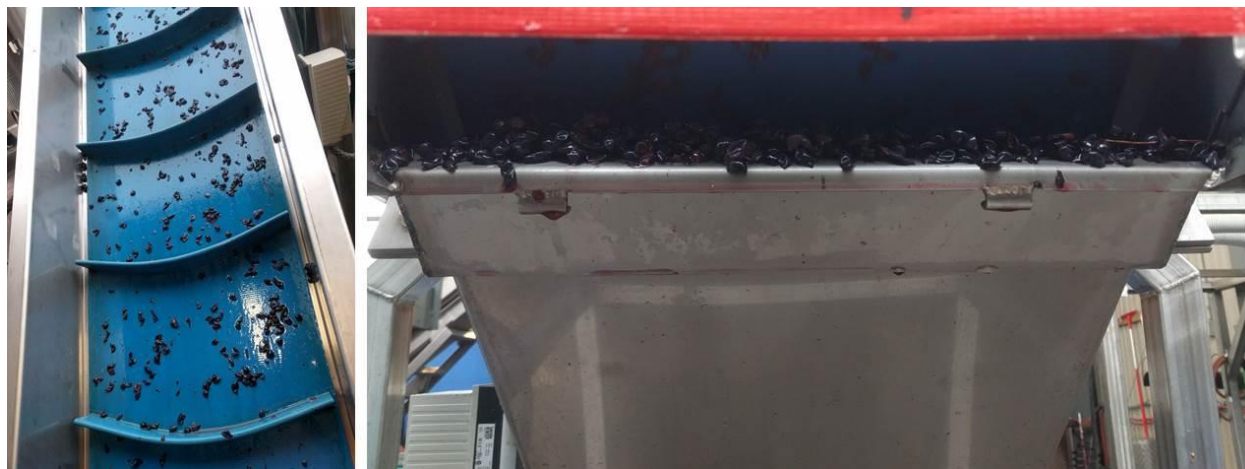
Figure 4. Grape material left on the sorting line after the machine was turned off.
